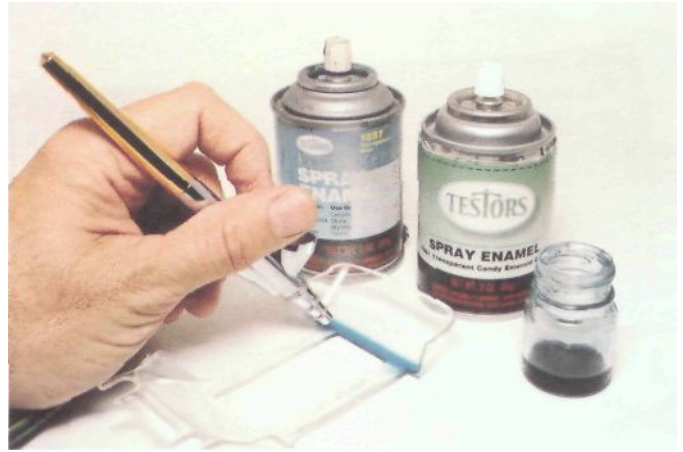
Fig. 4-4. Painting the dark tint strip across the top of a windshield adds realism to any car model, it is easy to apply using an airbrush with a fine nozzle.
