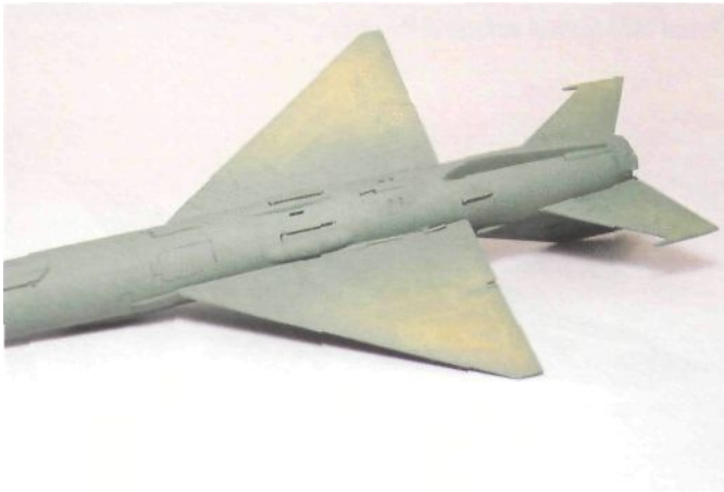
Fig. 12-2. Paint the undersides in metalizers (similar to the previous project, the all-metal version). Then mask these sections, as shown here, before painting the model pale green.
