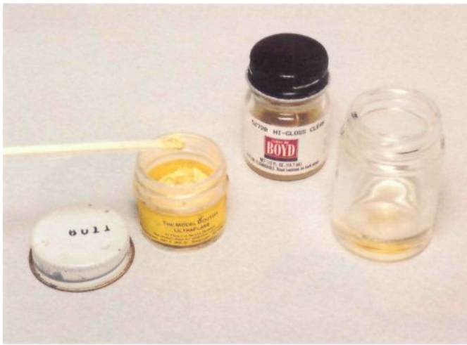
Fig. 8-8. Mixing the pearl into the paint is easy—just add a pinch of pearl powder to clear enamel.
