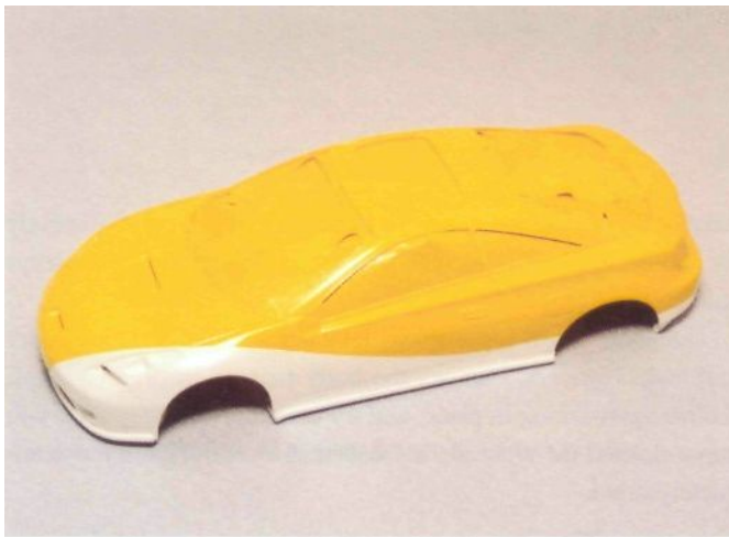
Fig. 8-10. Here are the finished yellow areas, after the masking has been removed.
