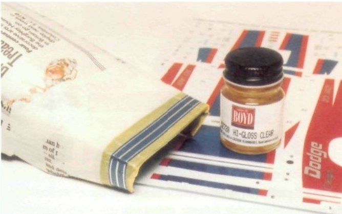
Fig. 10-8. Using photos or decals as reference, thoroughly mask the stripe area to be painted with a combination of Bare Metal Foil and Tamiya or similar brands of masking tape. To ensure none of the stripe color bleeds through, first spray a coat of clear over the masks. Any paint that does bleed through will be clear, nearly invisible, and easily polished smooth.
