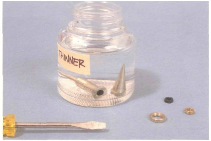
Fly. 1-22. Remove any rubber seals before soaking airbrush parts in thinner or other cleaning solvents. Kalmbach photo
