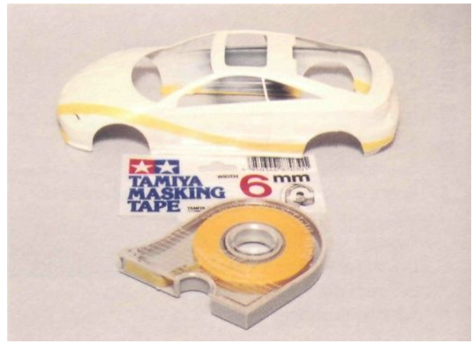
Fig. 8-4. Use Tamiya masking tape for clean color separation lines and overall ease of use.
