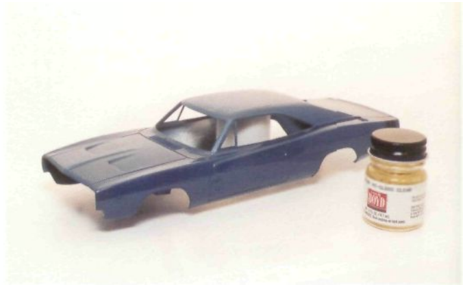
Fig. 10-13. The body is now covered in a uniform coat of clear gloss and is really looking good. When it is thoroughly dry and polished, it is ready for the vinyl top color. If you hold the body up to a light, you should be able to see the overlapping vinyl top, ready to paint.
