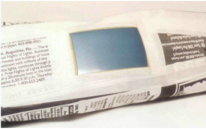
Fig. 10-12. After clear-coating the entire body, remove the center mask and let the clear coat dry thoroughly. Then, remask the body to add the overlapping center section of the vinyl top (as seen here), Paint the center section liberally with the same clear gloss mixture. When it has dried for about 30 minutes, you can carefully remove the masking.
