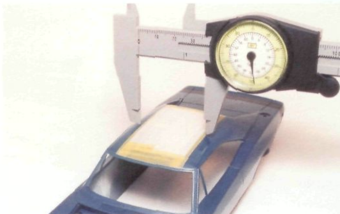
Fig. 10-11. Using photo references or another model to duplicate, carefully measure, cut, and apply a center mask for the vinyl top. Make sure the lines of the mask are parallel and centered on the roof, You can replicate the overlapping seams visible on a vinyl roof by overlapping the clear gloss coats in two steps. In the first step, mask the center of the roof, then coat the entire body with several coats of clear. Make sure to apply the final clear coats liberally, especially onto the roof area. This will give the seams added depth,
