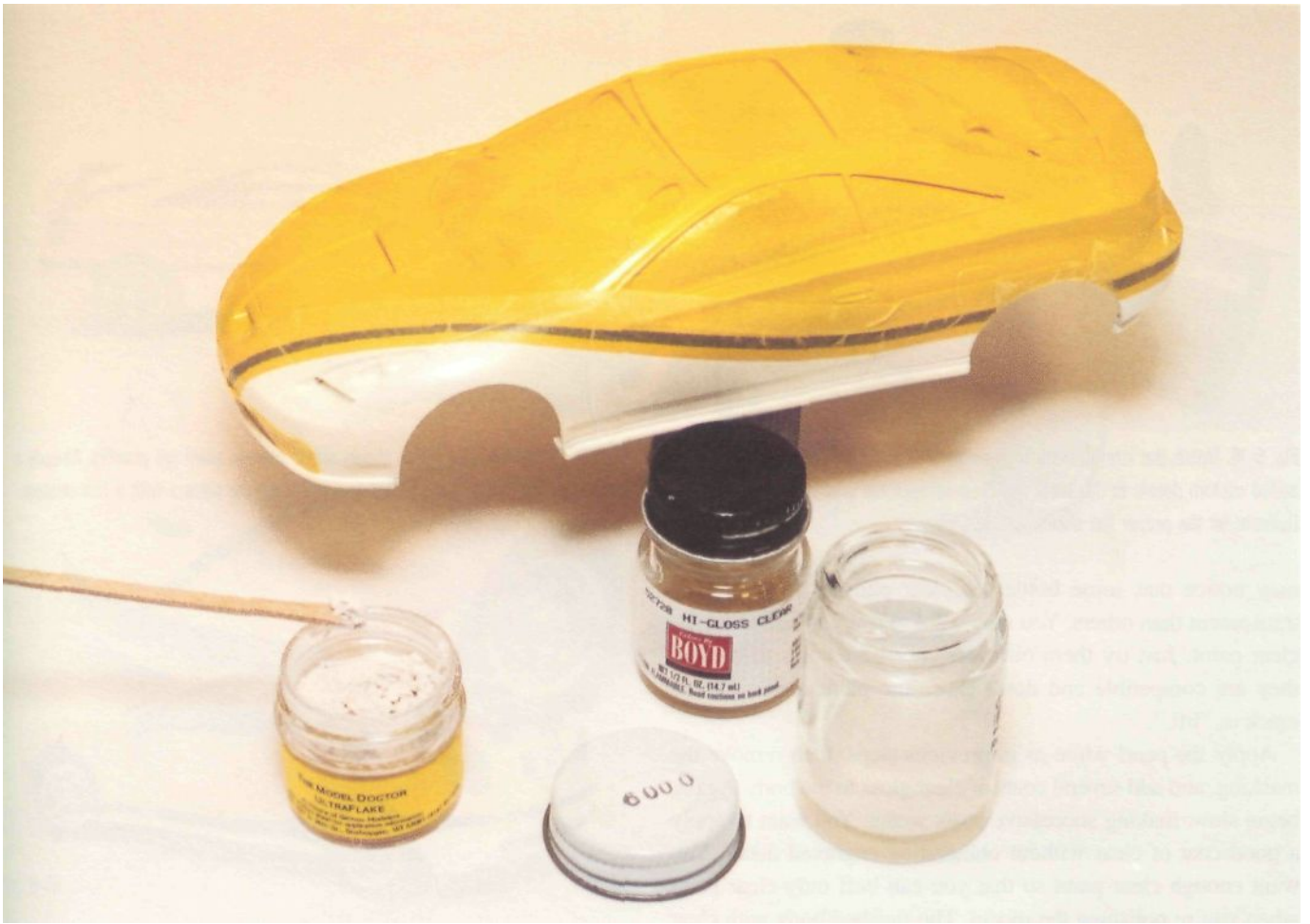
Fig. 8-13. The lower portion of the body, ready for pearly white paint. Add a pinch of pearl powder to some clear; it will cover rapidly with your airbrush.
