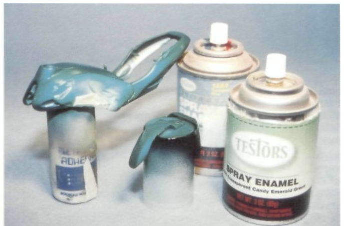
Fig. 9-12. Use cans of Testors Transparent Blue and Candy Emerald Green for the airbrushed color coats on the fenders and tank. Spray the colors into a glass jar first, then transfer and spray the mixture through your airbrush,
