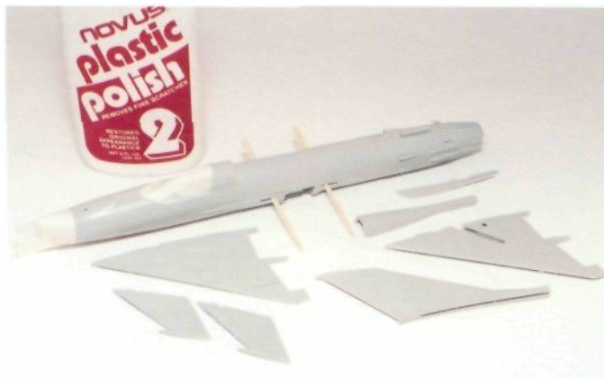
Fig. 11-4. A glossy finish for the metalizers requires a smooth, polished surface to work on. Buff these parts with Novus no. 2 plastic polish before airbrushing the metalizers onto the surfaces.
