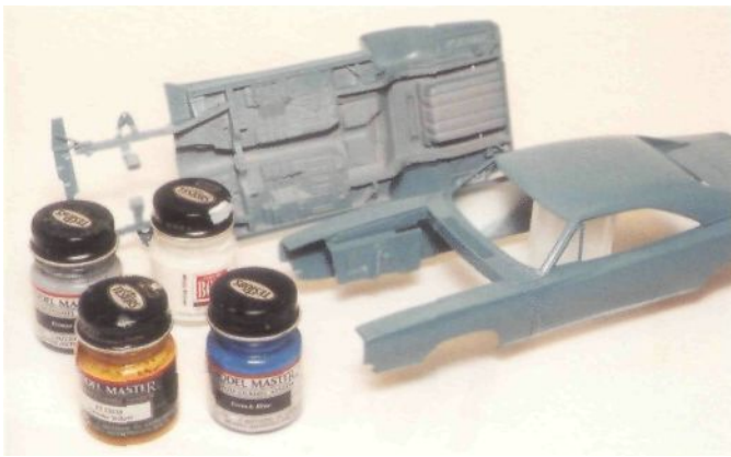
Fig. 10-2. To replicate the 1968 Charger Medium Blue Iridescent paint in enamels, begin with a solid-color basecoat that is similar to the final color. To create this result, add a mixture of Model Master French Blue and a few drops of Chrome Yellow to the gray/white primer mixture (from the previous step) for the basecoat, and spray it onto the model in several coats.
