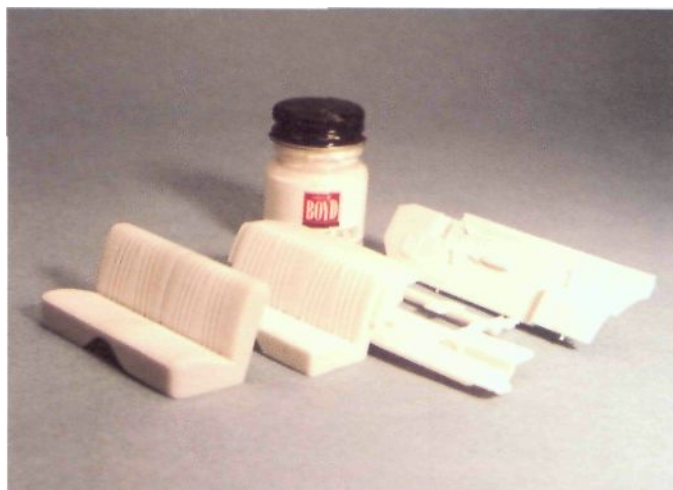
Fig. 6-1. Prime the basic interior components in white. Some of the white parts will be visible on the finished car.
