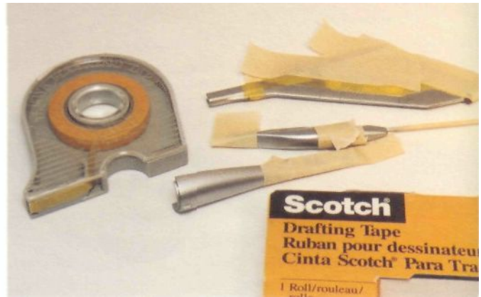
Fig. 11-16. You'll paint various sections in Nonbuffing Aluminum. Mask them, spray them with the metalizer, and seal them again with Gunze Clear acrylic.
