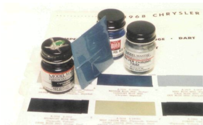
Fig. 10-5. If possible, try to find a genuine factory color chip to help you match the original color accurately. Authentic, original color chips can be found at some automotive paint stores for newer cars and at swap meets and specialized vendors for older cars.
