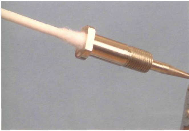
Fig. 1-21. Using a cotton swab dipped in thinner is a good way to clean the inside of the paint tip. Kalmbach photo
