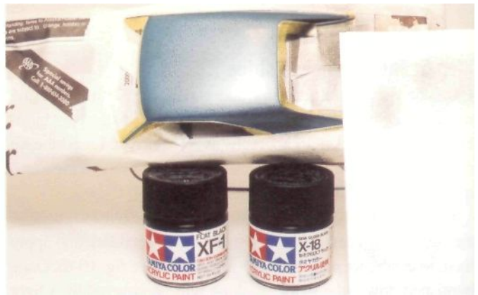
Fig. 10-15. Spray equal parts Tamiya Flat Black and Semigloss Black without thinner onto the roof. This will give you a nice, in-scale texture that accurately represents a vinyl top. Use a test card to practice spraying the texture seen here, before actually spraying your model. When you are comfortable with the texture and spray pattern, you are ready to paint the model,
