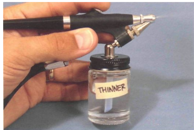
Fig. 1-20. Flushing your airbrush with fresh thinner after every painting session will make it easier to tear it down and clean it. Kalmbach photo
