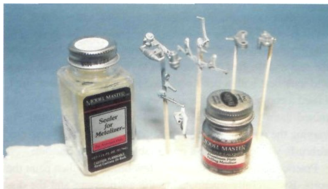
Fig. 9-8. Spray these chassis components with Aluminum Plate Metalizer and then seal them,
