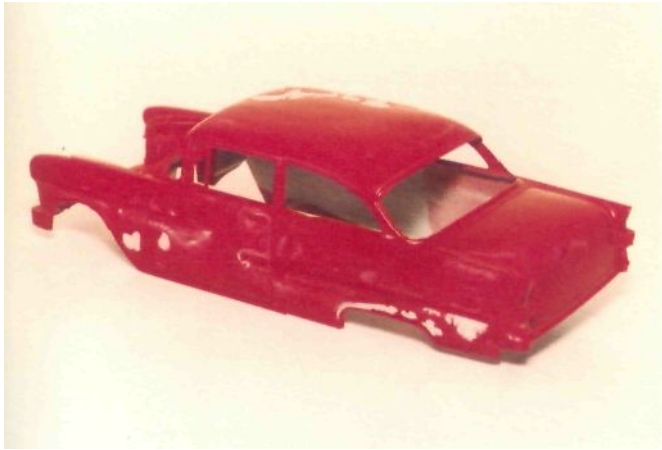
Figs. 1-29 and 1-30. Fisheyes (lack of paint adhesion) are caused by cleaning the surface of your model incompletely before painting.
