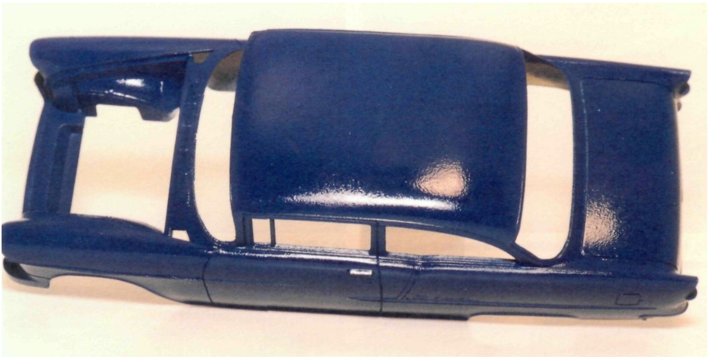
Fig. 1-28, An example of paint with an "orange-peel" surface. This is caused by not mixing enough thinner with the paint, or by using an inadequate airflow to propel the paint through the airbrush.
