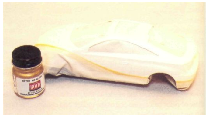
Fig. 8-6. Airbrush clear enamel onto the tape edges to prevent color bleed-through.
