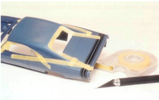
Fig. 10-14. Careful masking is needed to paint the vinyl top over the finished color coat underneath. Add the masking tape, burnish it, and use a fresh no. 11 blade to trim the edges accurately. Make sure the top area is clean of any fingerprints or polishing residue to avoid any potential problems with the vinyl top color. It's a good idea at this point to seal the edges with clear (as you did earlier with the bumblebee stripe, see (fig. 10-8) to avoid color bleed-through.
