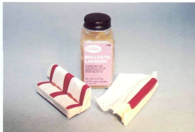
Fig. 6-4. You will paint several areas a dark shade of maroon. Carefully mask the previously painted areas as before, seal the edges with clear to avoid bleed-through of the colored paint.
