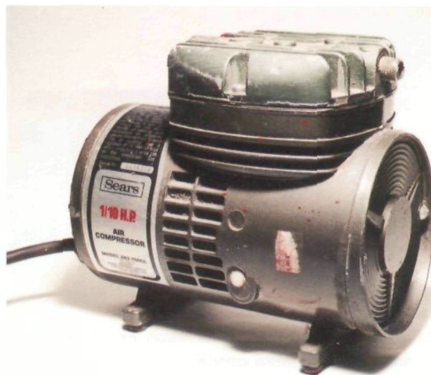
Fig. 1-7. This Sears compressor is an example of many that are available on the market from varied sources. Like all hobby compressors, it is an oil-less design, providing a stream of clean air to propel the paint.
