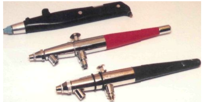
Fig. 1-2. Here are three common internal-mix airbrushes: a Testors/Aztek Model Master brush, a Paasclie VL, and a Badger Crescendo. All three provide good performance and control, and parts are readily obtainable.
