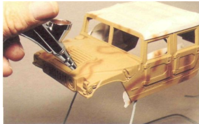
Fig. 3-2. You can add the camouflage pattern freehand with a fine-detail airbrush. Notice how close you can get to precisely "draw" the camouflage outline directly onto the model.
